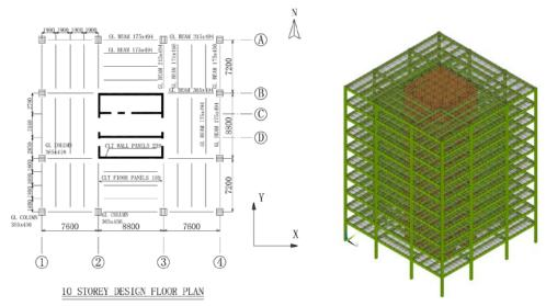
Figure 3. Designed structure and finite element model (Yang et al. 2018).
