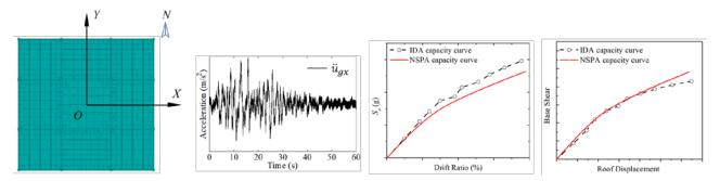
Figure 1. Footprint of a symmetric structure and schematic representation of capacity curve for unidirectional ground motions (the capacity curve is expressed in terms of SA versus drift ratio or Base shear versus roof displacement).
