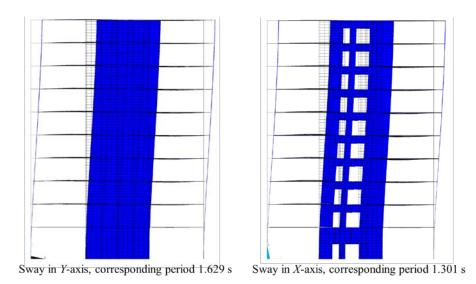
Figure 4. First two sway vibration modes.
