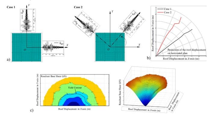
Figure 2. Illustration of capacity surface for a structure subjected to bidirectional ground motion: a) illustration of bidirectional ground motion, b) projection of the structural top displacement on the horizontal surface, c) Contour plot of capacity surface in terms of base shear, d) Surface plot of the capacity (capacity surface).
